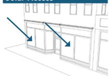
Awnings can be closed in the winter to provide solar heat gain and daylighting.
