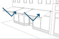
Awnings can be opened in the summer to provide shading for a storefront and the sidewalk.
