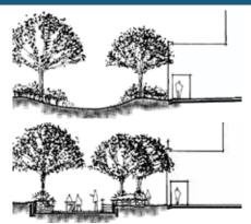
The design guidelines promote using LID principles to integrate stormwater management systems with public open space areas. The stormwater treatment areas illustrated above serve as a passive landscape amenity (top) and an outdoor seating area with a permeable surface (bottom).
