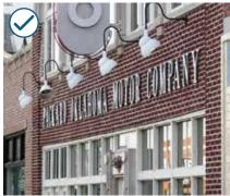
Locate a flush-mounted sign to fit within a panel formed by moldings or transom panels.
