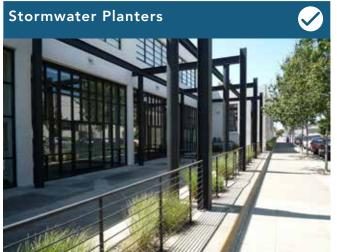
A stormwater planter is a specialized planter system installed adjacent to a sidewalk to manage street and sidewalk runoff. The planter is lined with a permeable fabric, filled with gravel or stone, and topped off with soil, plants, and sometimes trees.
